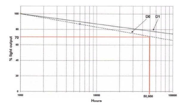
Lumen Maintenance For CR63RGB Per LRC LED Life Test Vol1 (ENG1210 and 1221)
